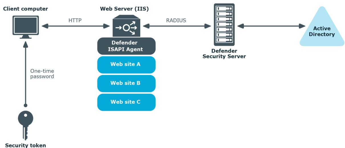
In this scenario, the Defender ISAPI Agent must be deployed on the Web Server that hosts the Web sites to be secured with Defender. The ISAPI Agent acts as an ISAPI filter and requires users to authenticate via Defender in order to get access to the Web sites hosted on the Web Server.
