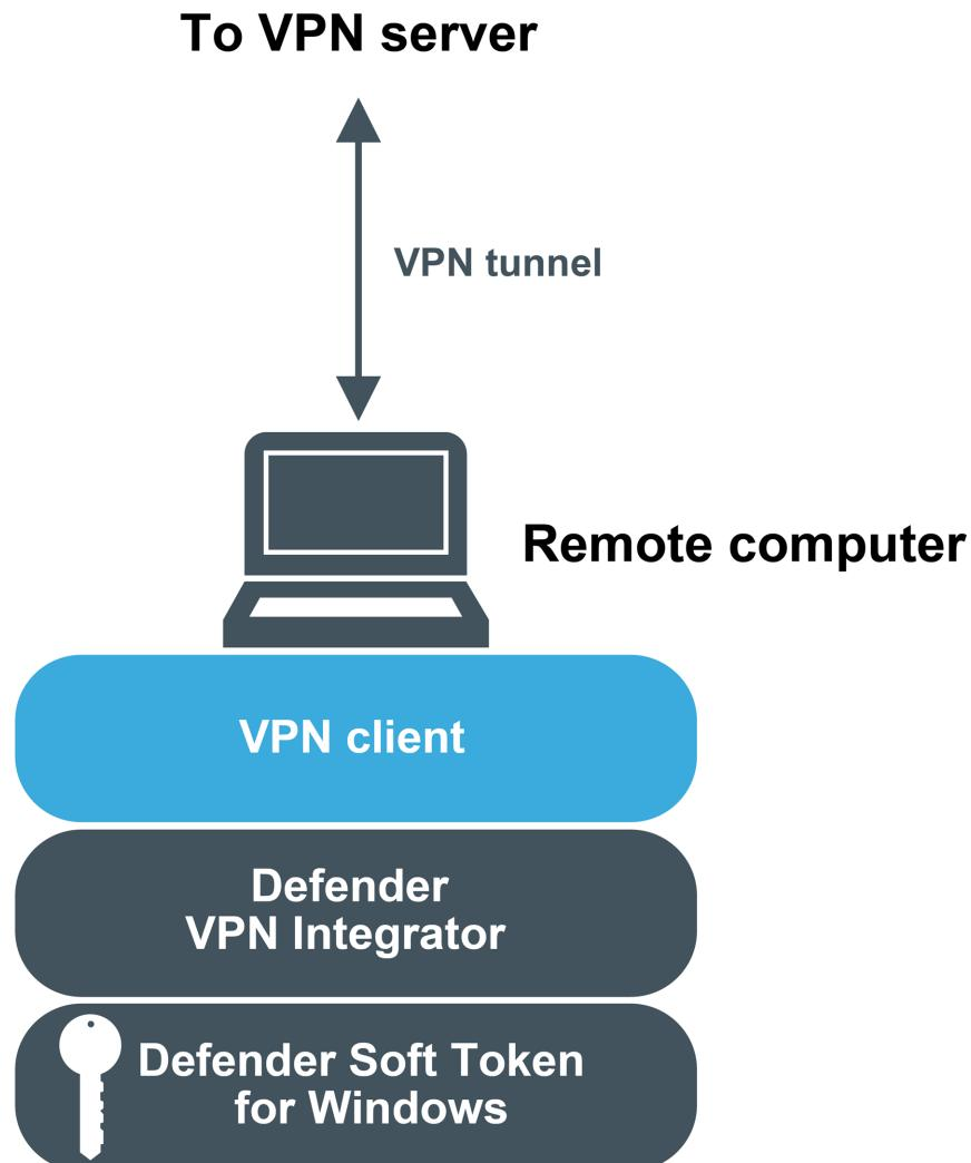
To do so, you need to install the Defender VPN Integrator on the computer where the Soft Token for Windows is installed. When the user initiates a VPN connection, VPN Integrator communicates between the Soft Token for Windows and the third-party VPN client to ensure that the secure, one-time password authentication process is handled.
