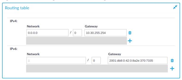
When sending a packet to a remote network, SPS consults the routing table to determine the path it should be sent. If there is no information in the routing table then the packet is sent to the default gateway. Use the routing table to define static routes to specific hosts or networks. You have to use the routing table if SPS interfaces are connected to multiple subnets.
