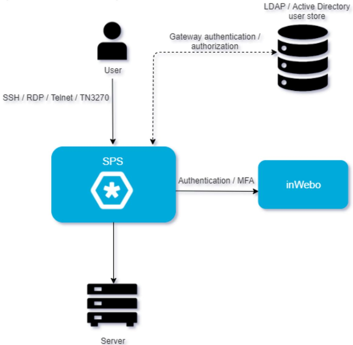
If SPS is integrated with inWebo, the interaction of the two products consists of the following steps:
