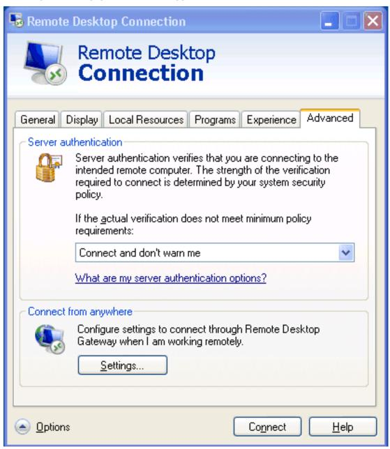
Configure the client to use SPS as its Remote Desktop Gateway. Select Connection settings > Use these RD Gateway settings.
