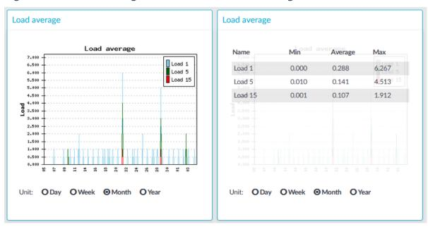
The **Load average** module on the **Dashboard** is based on data provided by the Linux kernel (/proc and /sys directories). The standard Munin plugins query this information from these locations and they are displayed on the GUI.
