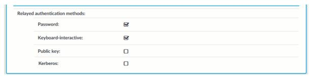
• **Password**: Authentication based on username and password. The server will request a password from the user, even if a password-based authentication was already successful on the client-side.
