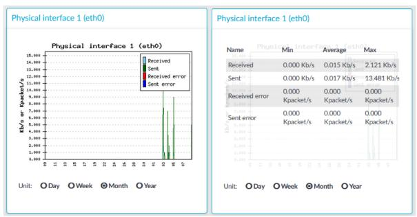
The **Interface** module on the **Dashboard** is based on data provided by the Linux kernel (/proc and /sys directories). The standard Munin plugins query this information from these locations and they are displayed on the GUI.
