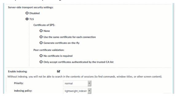
To require encryption, select **TLS**. When the connection is encrypted, SPS has to show a certificate to the peer.
