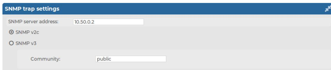
The screenshot shows the 'SNMP trap settings' configuration page. At the top, the title is 'SNMP trap settings'. Below it, the 'SNMP server address' is set to '10.50.0.2'. There are two radio button options: 'SNMP v2c' (which is selected) and 'SNMP v3'. Below these options, the 'Community' field is set to 'public'.
