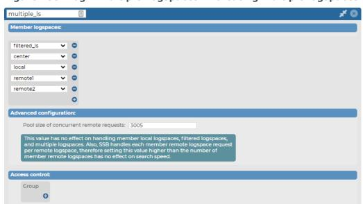
Figure 153: Log > Multiple Logspaces — Creating multiple logspaces
