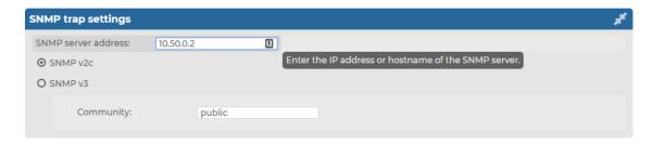
If you want to configure SNMP v3 trap settings, select **SNMP v3**, provide the SNMP server address, the **Username** and the **Engine ID** you want to use, then configure the **Authentication method** and **Encryption method**you want to use.
