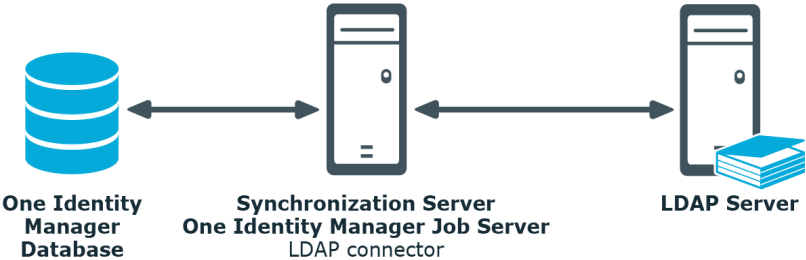
Figure 1: Architecture for synchronization
