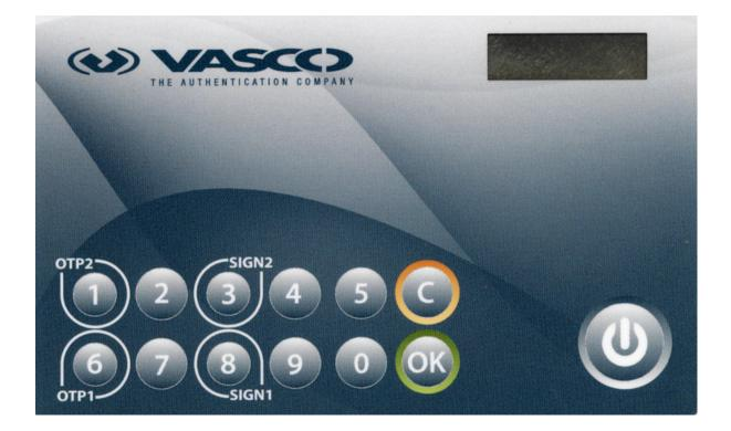
To authenticate and access resources protected by Defender, use the one-time password (OTP) application of the DIGIPASS 280 token (the OTP1 and OTP2 buttons). Currently, Defender does not support the e-signature application of the token (the SIGN1 and SIGN2 buttons).
