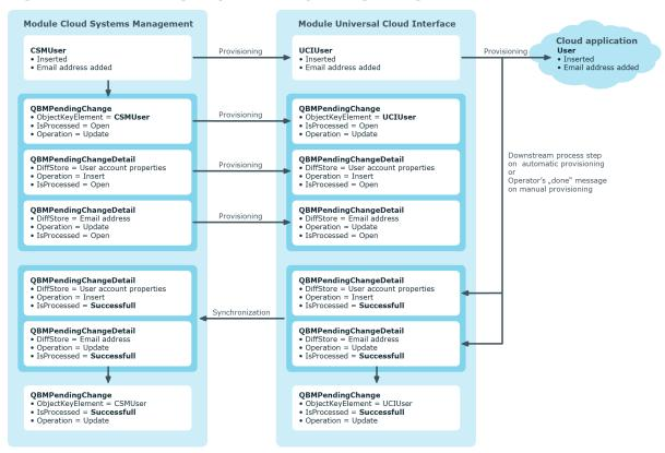
Figure 3: Provisioning sequence for pending changes
