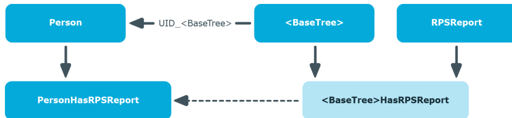
Figure 3: Inheritance with indirect primary assignment of software to employees
