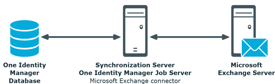
Figure 1: Architecture for synchronization
