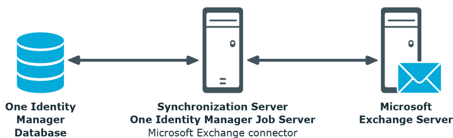
Figure 1: Architecture for synchronization
