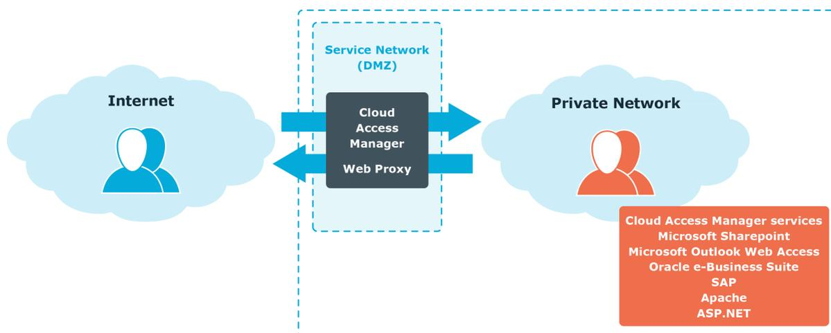
In addition to providing URL-based access control to firewalled applications, the web proxy also protects Cloud Access Manager web components such as the Security Token Service (STS) login pages, application portal and administration interface. The web proxy enforces authentication and authorization policies to applications running on the trusted network.
